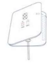
Step4: Peel off the adhesive, and fold the left side over, wait for 15 minutes.
